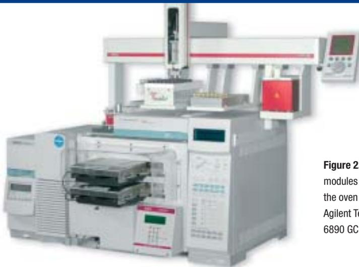
**Figure 2.** Two MACH modules installed in the oven door of an Agilent Technologies 6890 GC.
