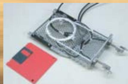
**Figure 1.** MACH GC Module based on Low Thermal Mass (LTM) technology (covers removed); Inside, the specially packaged column can be seen along with the heated transfer line connectors and high-temperature interface. The 3.5" Floppy Disk is shown for size comparison.
