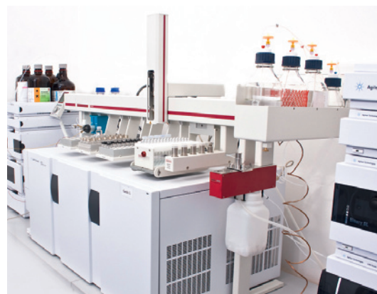
The SPE LC-MS/MS system used by the TeLA scientists for the pesticide multi-residue method consisting of an Agilent Series LC 1200 and a GERSTEL SPE system mounted over an Agilent 6410 MS/MS Triple Quad.
